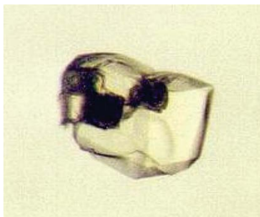
Figure 3 Photograph of a 400 \mu\text{m} neuramidase crystal (subtype N9 from avian influenza isolated from a noddy tern), space group I432 , that has been irradiated on ID14-4 at the ESRF at 100 K and then allowed to warm up to RT. The three black marks are from the 100 \times 100 \mu\text{m} beam; the discolouration is an indication of radiation damage.
